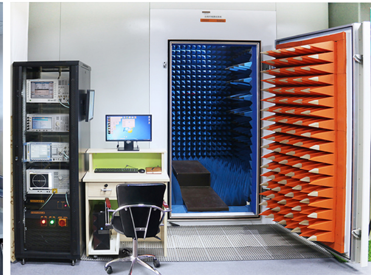
In-house Anechoic Chamber
